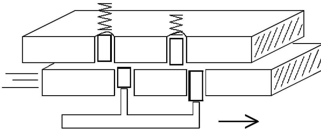
Figure 3.3: (b) Proper key allows plates to slide
