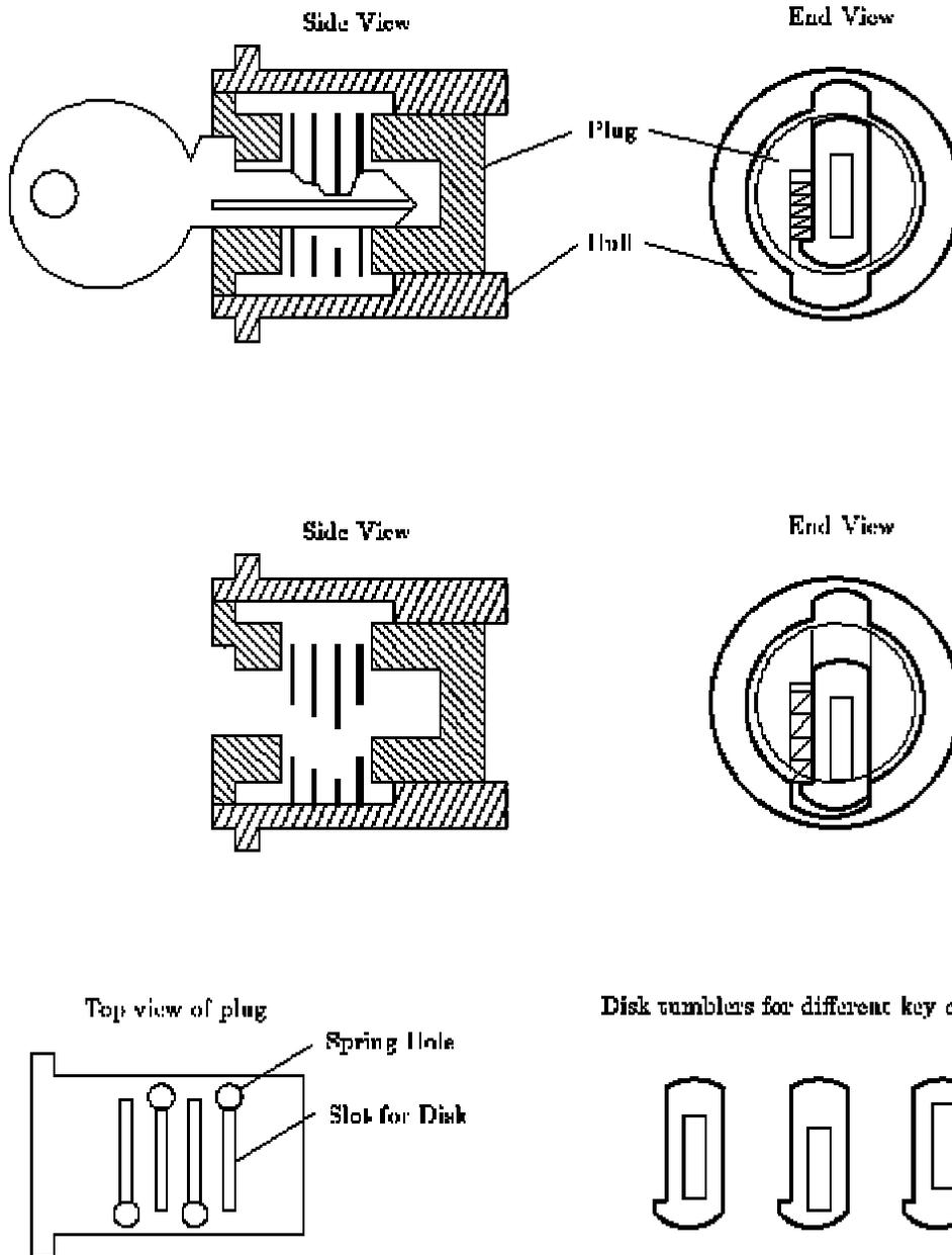
Figure 9.10: Workings of a disk tumber lock
