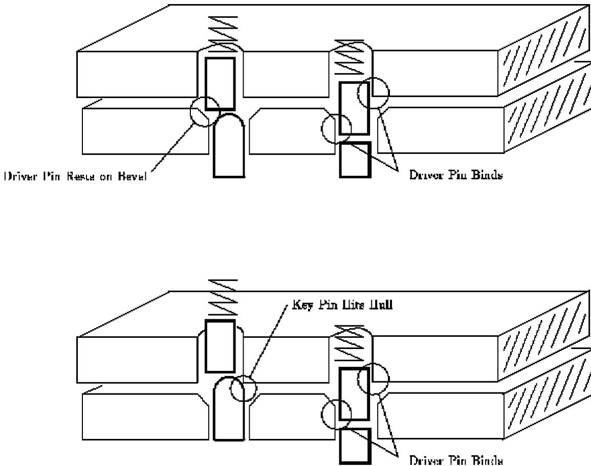
*Figure 9.4: Beveled plug holes and rounded key pins*
