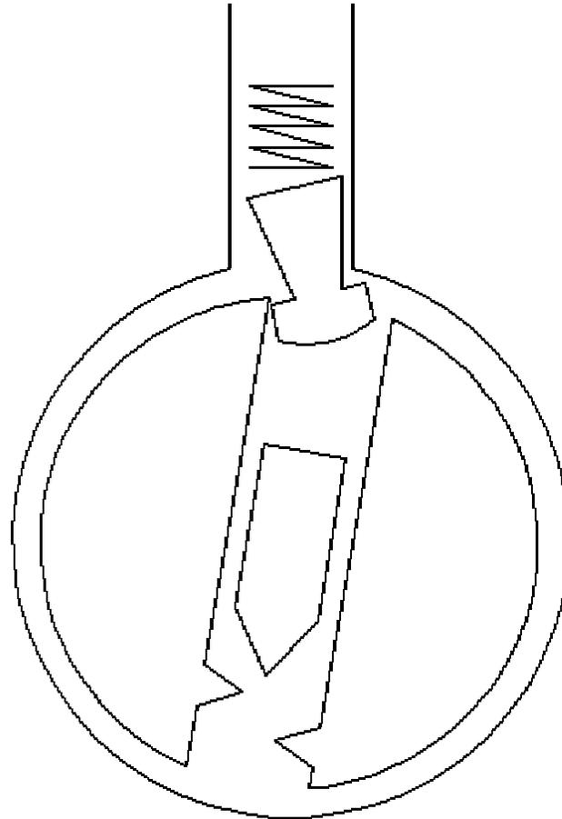
*Figure 9.7: Mushroom, spool, and serrated driver pins*
