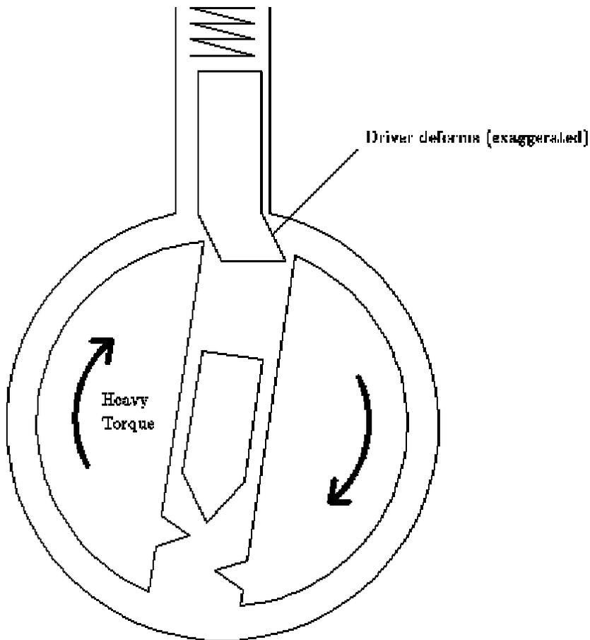
Figure 9.2: Driver pin false set by elastic deformation
