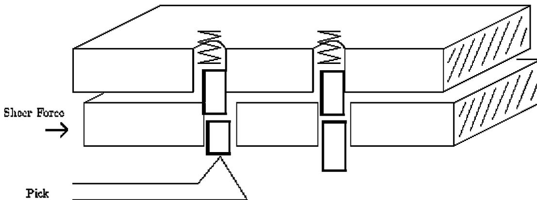
Figure 4.2: (b) Pick lifts the binding pin
