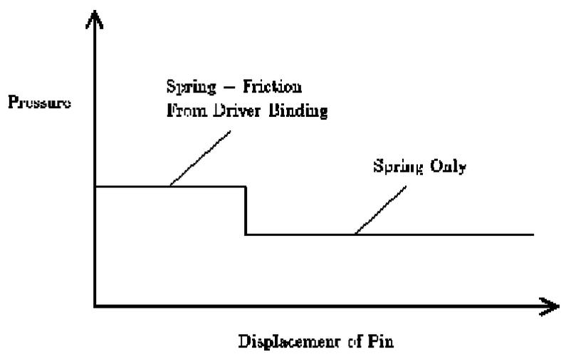
Figure 9.3: Driver pin wider than key pin
